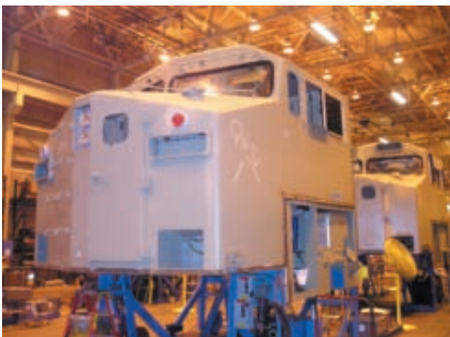
Cabin assembly line at GE's shops in Erie.
